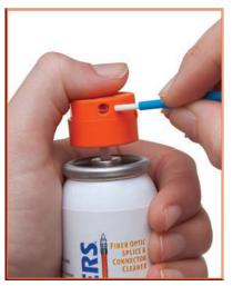
Use the Sticklers® Fiber Optic Splice & Connector Cleaner to dampen the Sticklers® CleanStixx™ Connector Cleaning Sticks
